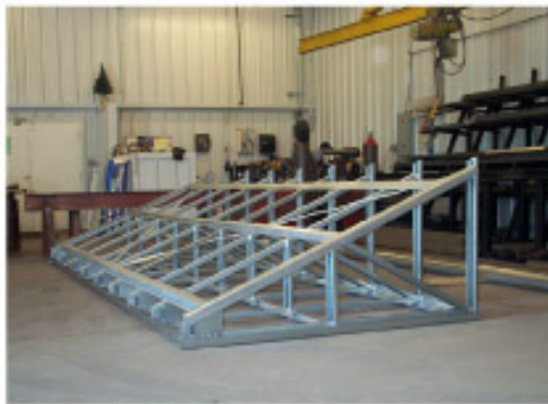
Shop assembled canopy framing system awaiting shipment from our fabrication facility. The finished canopy is shown below
